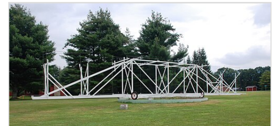
Reconstruction of the directional antenna used in the discovery of radio emission of extraterrestrial origin by Karl Guthe Jansky at Bell Telephone Laboratories in 1932
